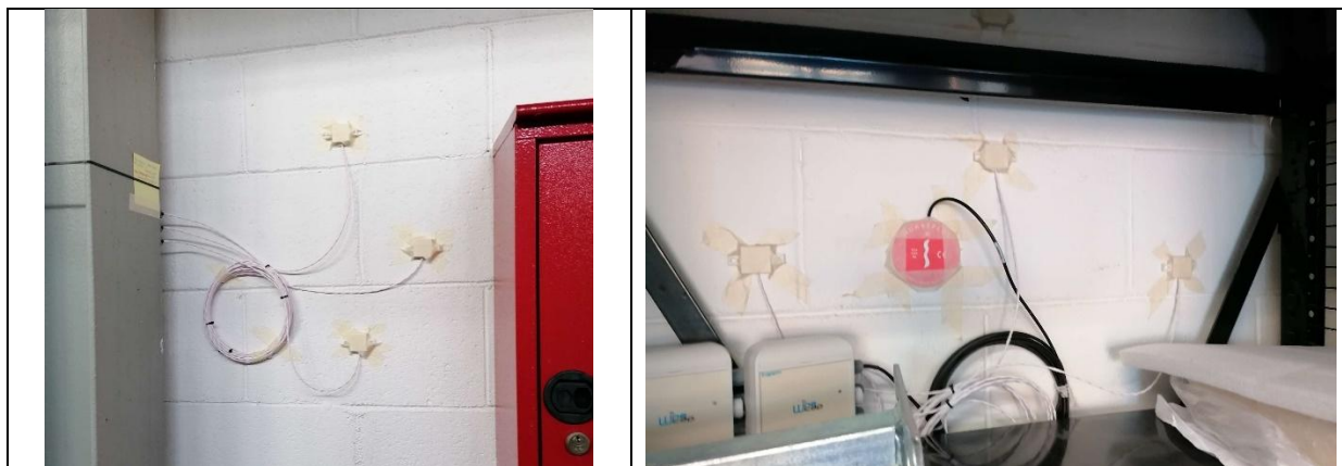
Figure 38 - the installed set of sensors to compute wall U-values
