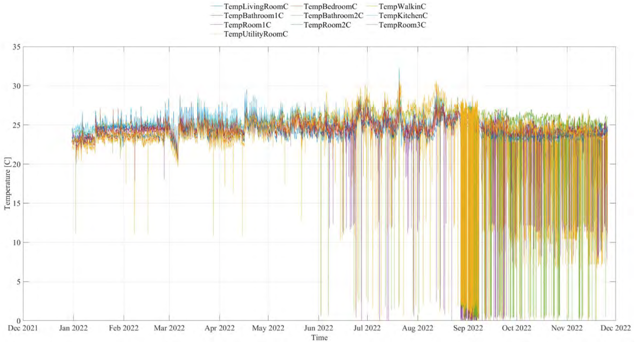
Figure 18: Data for temperatures in Ry demo case before outlier detection and data imputation.
