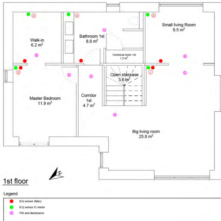
Figure 62: Location of the IC-meter IE sensors, the dismantled Niko Multisensors, and the Niko PIR sensors on the 1st floor. The letters in the circles are for data location Appendix C. Name for data location: Sensor_1st.
