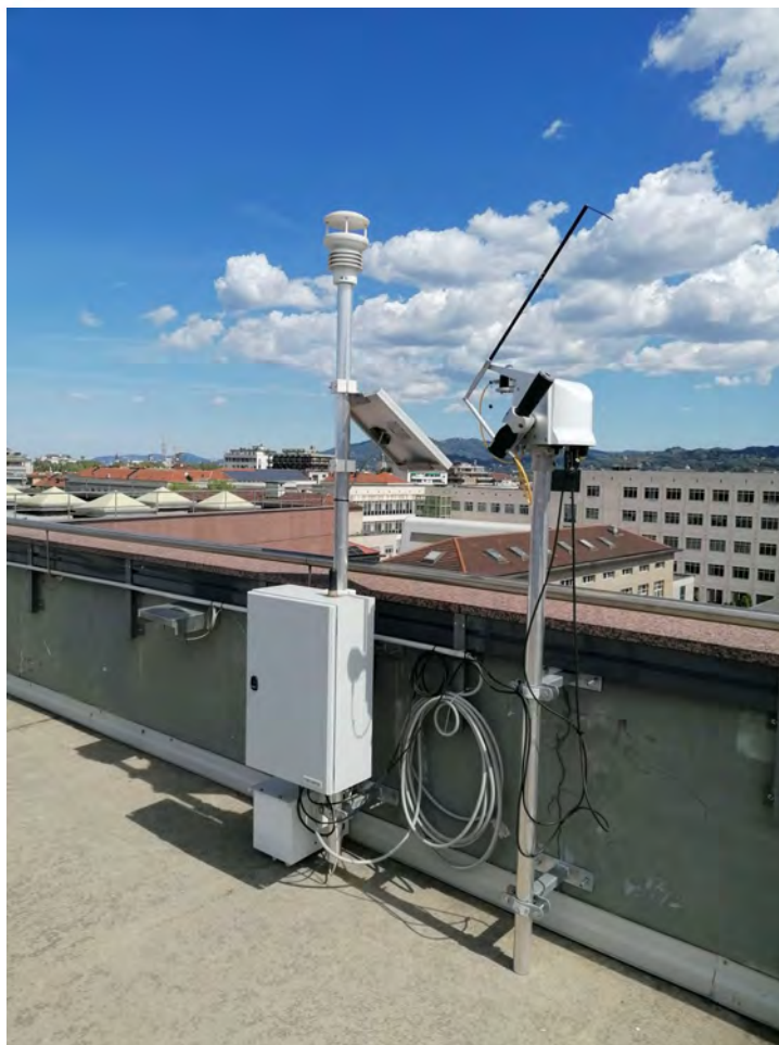
Figure 19- The installed meteorological station Exploratory analysis of occupancy profiles.
