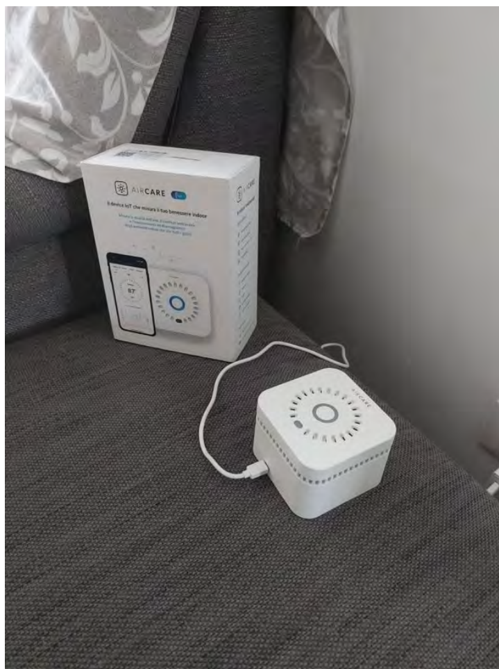
Figure 8 Indoor monitoring device AIRCARE installed in the demo site apartments
