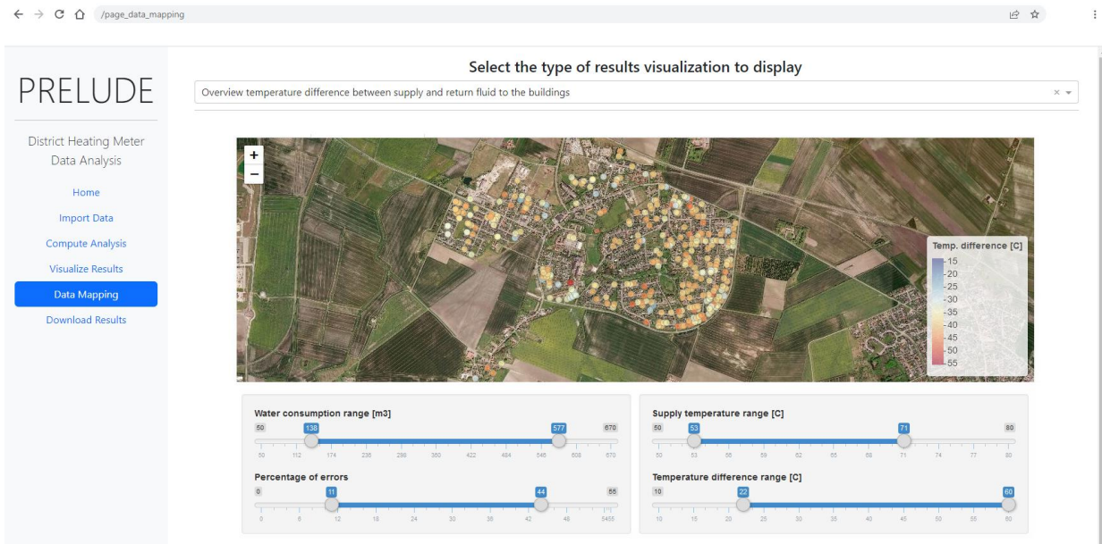
Figure 22: Example of Data Mapping: Overview temperature difference between supply and return fluid to the buildings of a town.
